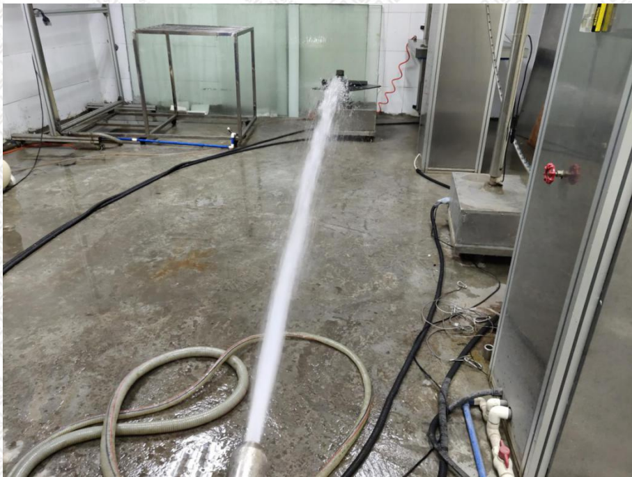
Photo 4: IPX6 test of model LT600+LT600B-76/LT600C-C1055
