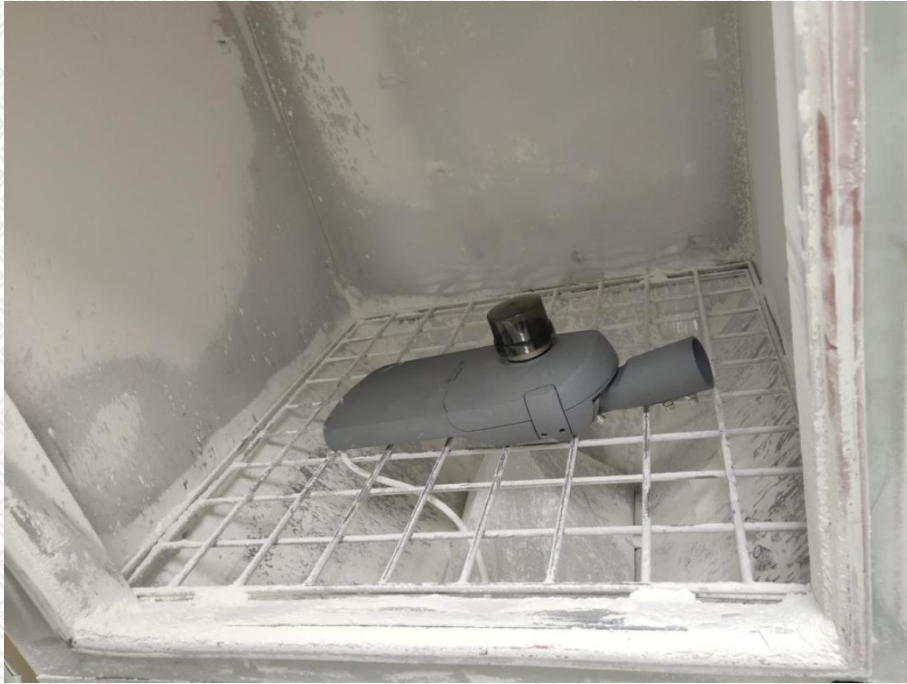
Photo 3: IP6X test of model LT600+LT600B-76/LT600C-C1055
