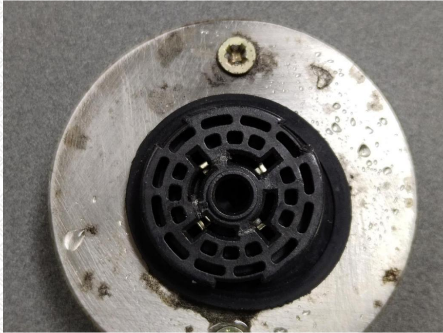
Photo 5: Test result after IP6X and IPX6 test
